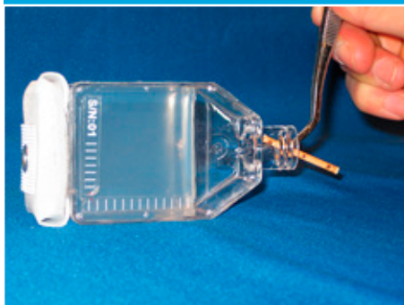
Demonstration of how an astronaut on the Space Station would insert a balsa wood strip with attached seeds into a prepared flask. Photo courtesy of BioServe Space Technologies.
