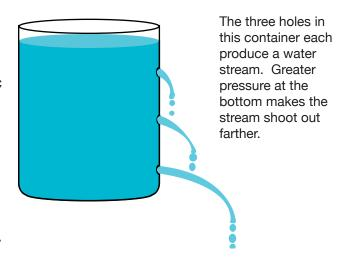
The effects of the other variables are many. For example, more holes means more water streams out of the can, but the water drains from the can more quickly. Large holes drain water more quickly than small holes. Holes angled in different directions counteract each other. Holes that are not angled produce water streams that leave the can perpendicular and no rotation occurs. (The object is to have students discover the effects of the different variables themselves.)
