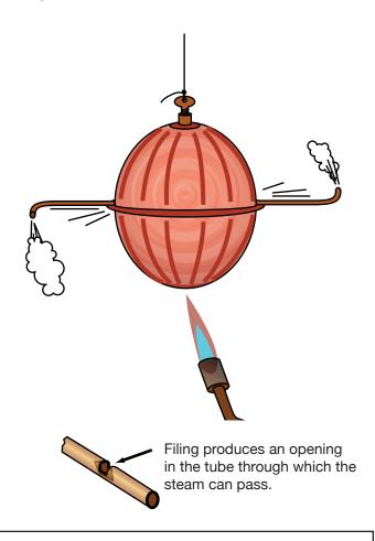
**Tip** Before using your steam Hero engine, confirm the tubes are not blocked by blowing through them. If air comes out the opposite tube, the engine is safe to use.
