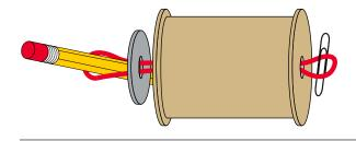
3. Slip the other end of the rubber band through a washer. Then slide the pencil through the rubber band loop (see illustration above). The spool racer is ready for testing.
