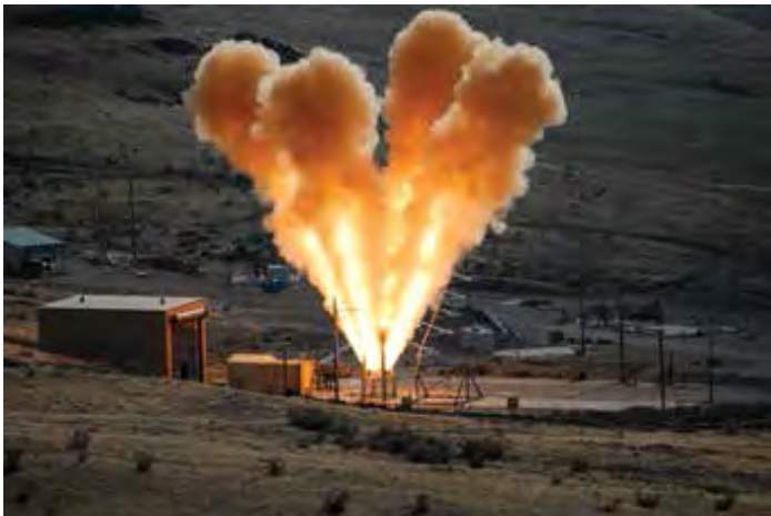
Static firing of the Orion escape rocket.
