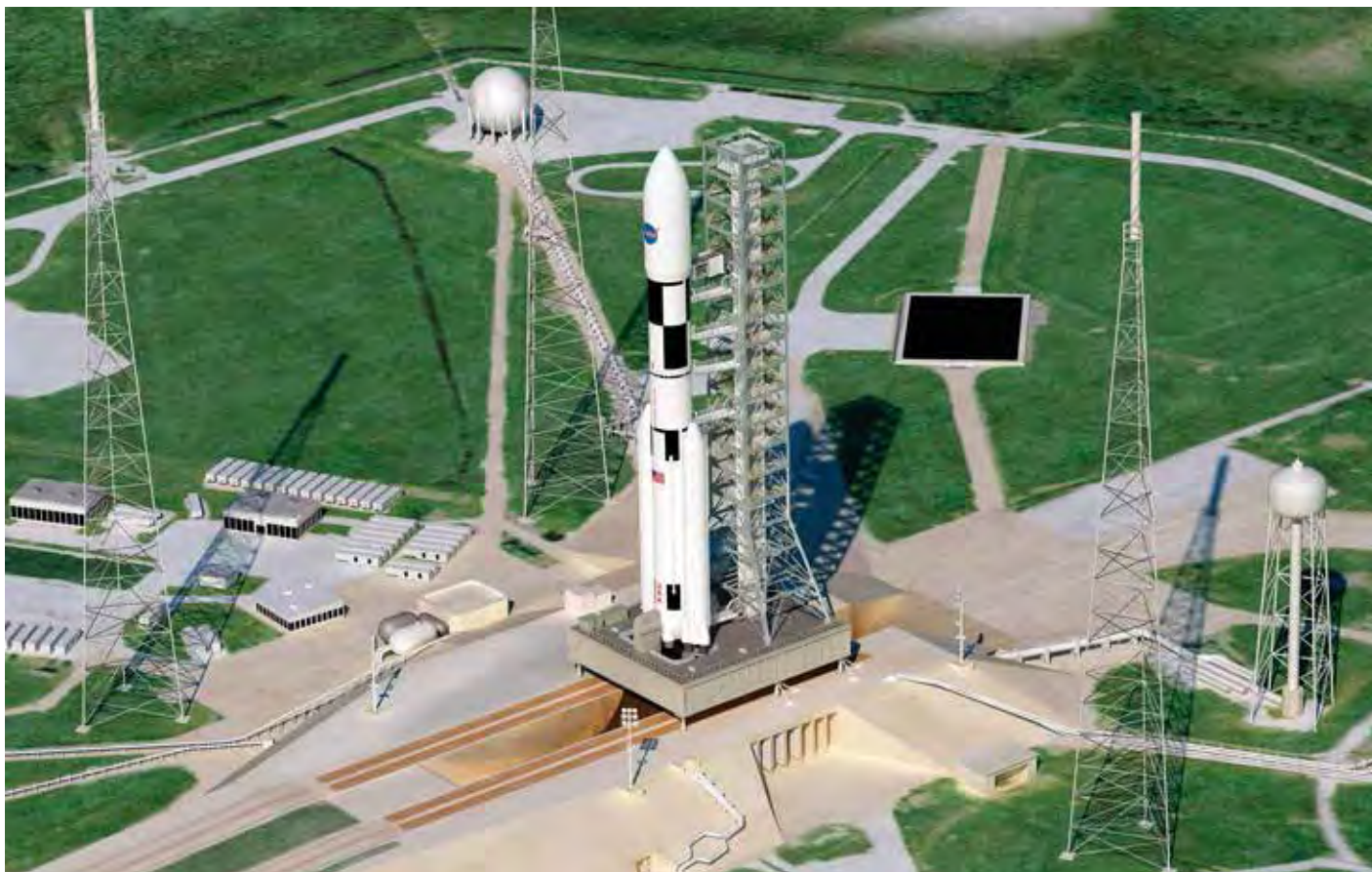
NASA's advanced SLS rocket will stand 122 meters (400 feet) tall, with a lift capacity of 130 metric tons (286,000 pounds). Here it is shown configured to carry cargo.
