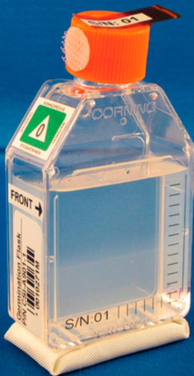
Germination flask containing two different densities of media, ready for delivery to NASA for transport to the International Space Station (ISS). The higher density layer of growth media used in the ISS experiment is visible about halfway down the flask.
