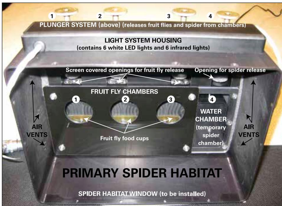
BioServe Commercial Generic Bioprocessing Apparatus (CGBA) on the ISS. The CGBA will power the habitat lights and cameras, and will maintain the correct temperature (25°C) for the habitats.
