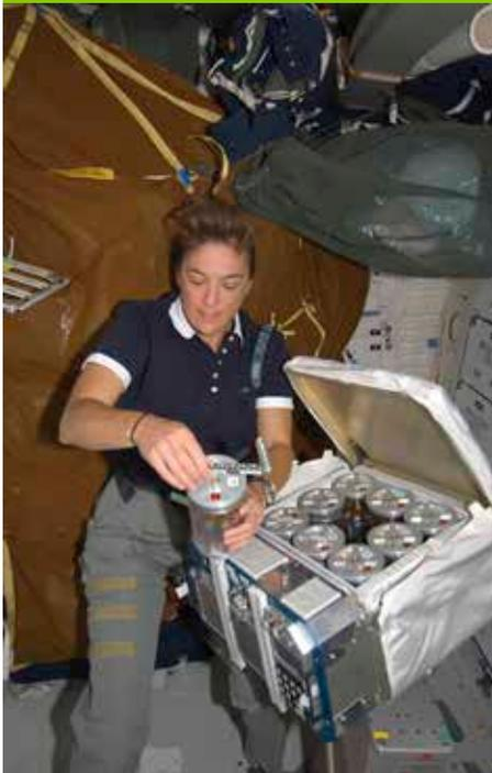
Mission Specialist Heidemarie Stefanyshyn-Piper (STS-126) works with a customized, temperature controlled experiment insert, part of the Commercial Generic Bioprocessing Apparatus (CGBA) on the middeck of Space Shuttle Endeavour, while docked with the International Space Station. Photo courtesy of NASA.
