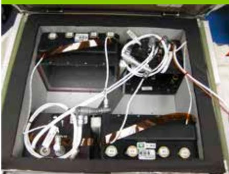
Top view, inside a CGBA insert housing small spider habitats (upper left and lower right) and cameras, part of Mission STS-134. Photo courtesy of BioServe Space Technologies.
