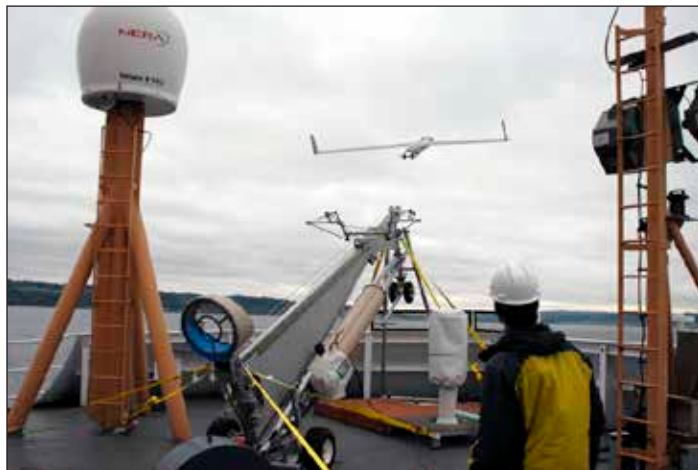
NOAA uses a pneumatic catapult to launch the ScanEagle, an unmanned monitoring aircraft.
