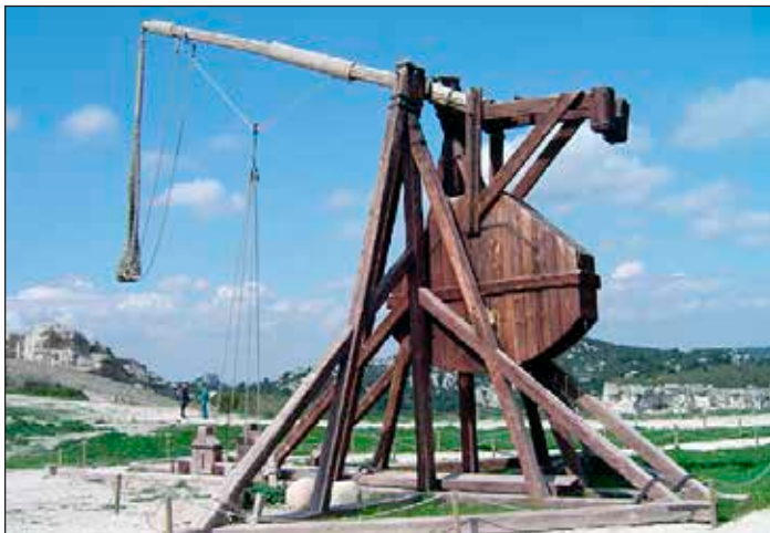
A trebuchet catapult used a raised counterweight and a sling to send huge stones or incendiary ammunition over or through walls. Shown above is a Medieval trebuchet in Château des Baux, France.
