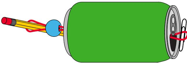
3. Push the end of the rubber band through the hole in the can bottom. Using the paper clip hook, reach inside the top of the can and capture the loose end of the rubber band.
