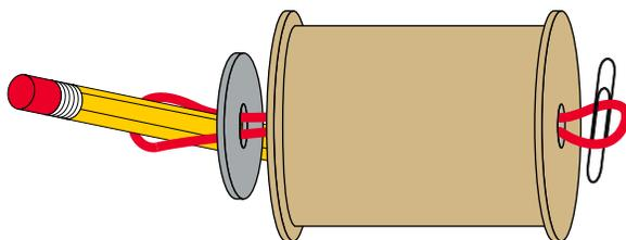
3. Slip the other end of the rubber band through a washer. Then slide the pencil through the rubber band loop (see illustration above). The spool racer is ready for testing.
